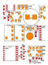
optimise the amplitude of the if filters, but not the phase response. It is a good idea to adjust the filter matching by observing the eye pattern at the receiver output. While receiving a 153 kbaud signal, you watch the eye pattern and adjust L665 and L682 for optimal symmetry and eye.
