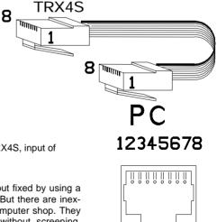
RJ-Connector, rear view. Only pins 3,4,5 and 6 are used The cables are available as: 8-wire flat cable / modular-cable with rj45 connector, ISDN-cable rj45, patch cable 1:1 connected, cable with 8 pin western-connectors. If you find similar cables with smaller 6 or 4 pin connectors, as used with other telephone applications, you may use them as well. Screened cables are much more expensive, but provide better suppression of radio interference.
