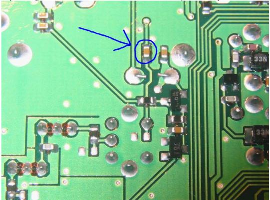
Location of the chip capacitor C3371 on the chip side of the printed circuit board
