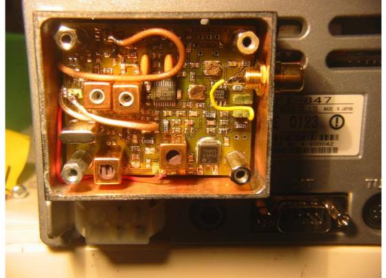
22. Use a 10 mm M3 screw in the bottom holes and install a 4mm hex nut spacer inside the box. Then install the IFD in the box and fix it with 4 15mm spacers. The cover of the box can be fixed with 4 screws which fit into these long spacers. It is necessary that the length of the spacers and the height of the case match exactly. If the spacers would be too long, there is a bad gap between case and cover.
