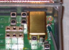
7. Now carefully fold the board to left. All cables may remain connected. Under the brass shielding box locate the C3371 SMD capacitor and remove it. It is glued to the board so you have to heat it and push until the glue releases the part. The IFD has to be inserted in the 50 Ohm signal path between the balun output and the resonant transformer circuit. Remove simply the coupling capacitor C 3371 (10 nF) and connect a 50 ohm coaxial to each end of the removed capacitor.
