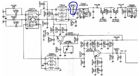
Here you see the transceiver front end: left side the balanced mixer, middle the balun with its 50 Ohm output and right the transformer which matches the 50 Ohm to the quartz filter input.
